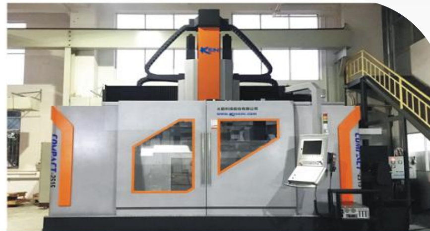
5-axis TCH-19(A63) CNC Machining: 1set Major Parameters: 2500x1500x1000mm
