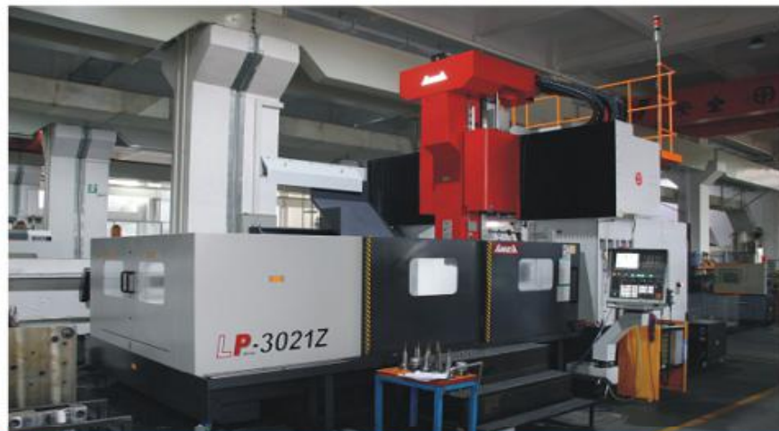
AWEN Numerical high speed milling machine: 2sets Major Parameters: 3000x2000x1000mm
