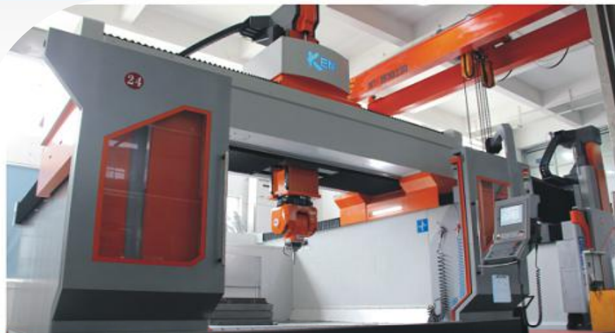
5-axis TCH-19(A63) CNC Machining: 1set Major Parameters: 3200x2200x1250mm
