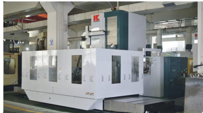
KURAKI KBT-13E CNC Machining : 1set Major Parameters: 3000x1600x760mm
